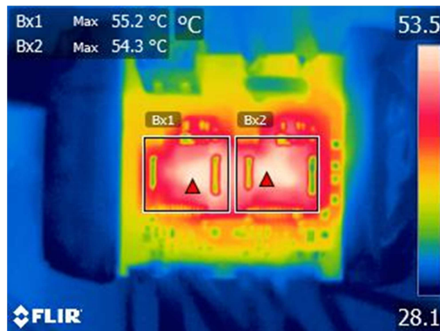
Figure 22 – Thermal Scan at 30 W Inverter Output in External-Supply Operation.
